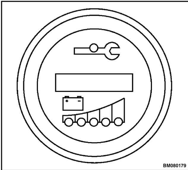
Figure 9. Battery Indicator/Hourmeter Display
